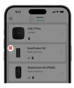
When a malfunction is detected, the Ajax app displays a malfunction counter on the device icon. All malfunctions are shown in the detector states. Fields with malfunctions will be highlighted in red.
