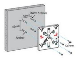
(2) Align the square feet on the rear of the AP with the mounting holes on the bracket.
