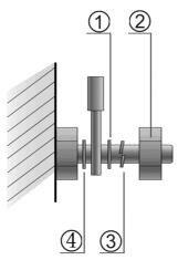
Note 1. Flat washer 3. Spring washer 2. Nut 4. Flat washer
