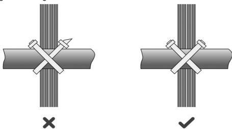
o If cables are to be bent, bind them first but do not tie cable ties within the bend to avoid stress on the cables, which may otherwise cause the wires inside to break, as shown in **Figure 7-6**.
